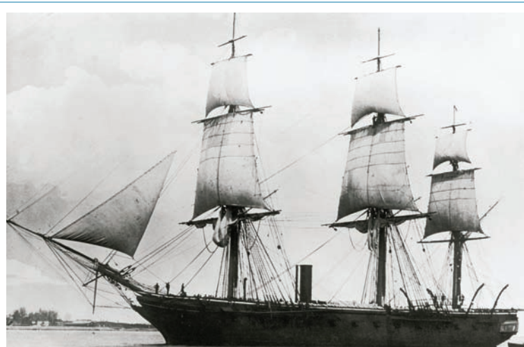
Early steam-powered warships still sometimes hoisted sails to supplement the steam engines.
